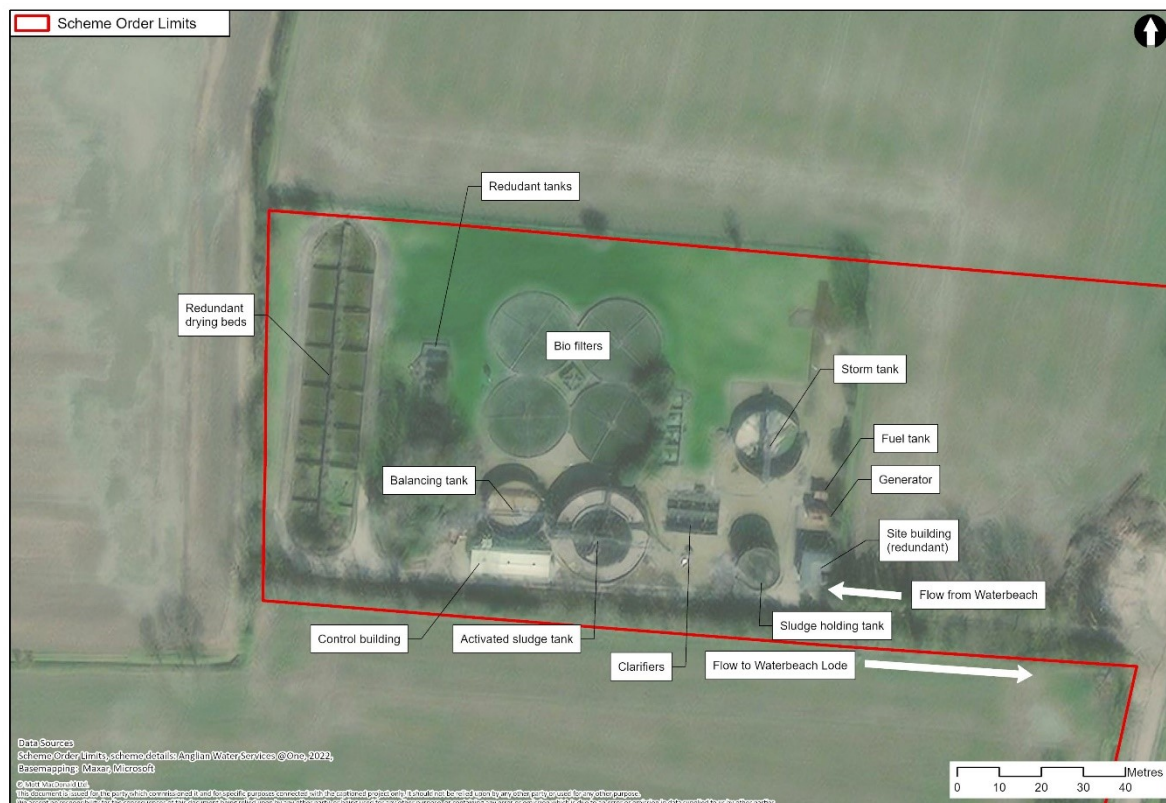
Figure 8.3: Schematic of the Waterbeach WRC
