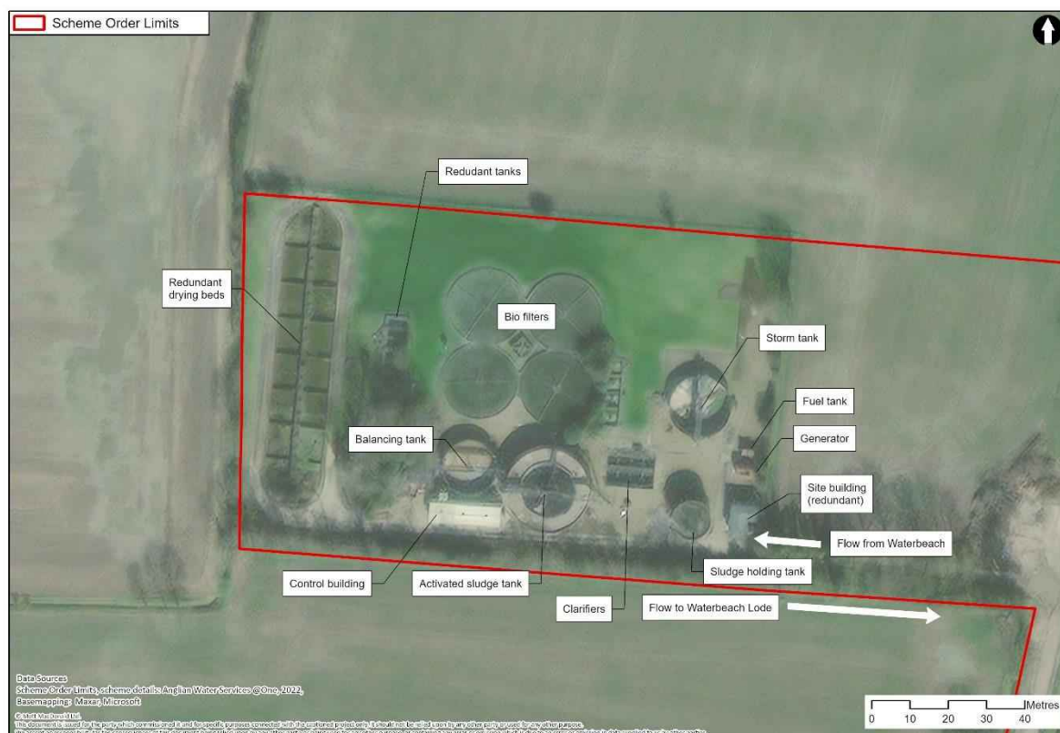
Figure 8.3: Schematic of the Waterbeach WRC
